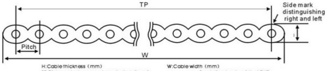
H:Cable Inickness (mm) IP:Distance between end conductors (mm) Notes:Side mark - Stranded: green Hi-warp:red
